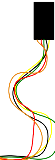
CN1 Connects to CN3 on MTX
