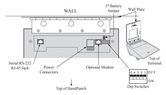
Figure 12-4: Wiring Connections and Dip Switches
