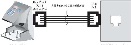
Modem Unit Figure 4-4: Host PC to HandPunch Modem Connection
