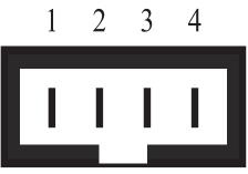
Figure 4-2: J4 - RS-232 Jack Pinout
