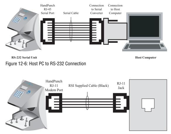
Modem Unit Figure 12-7: Host PC to HandPunch Modem Connection
