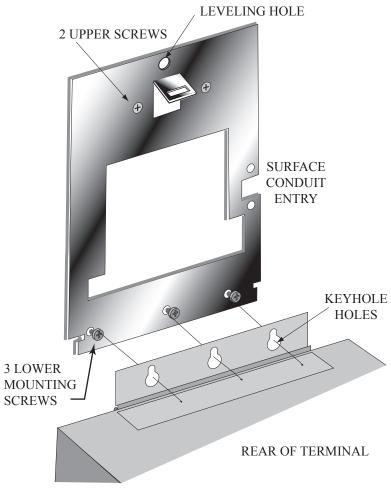
Figure 12-3: Attaching the HandPunch to the Wall Plate
