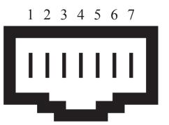
Figure 12-5: J4 - RJ-45/RS-232 Jack Pinout
