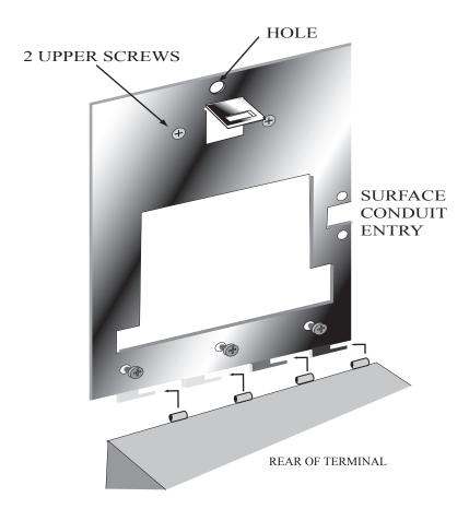
Figure 3-3: Attaching the HandPunch to the Wall Plate
