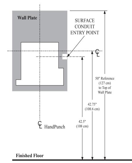
Figure 3-2: HandPunch Wire Routing Layout
