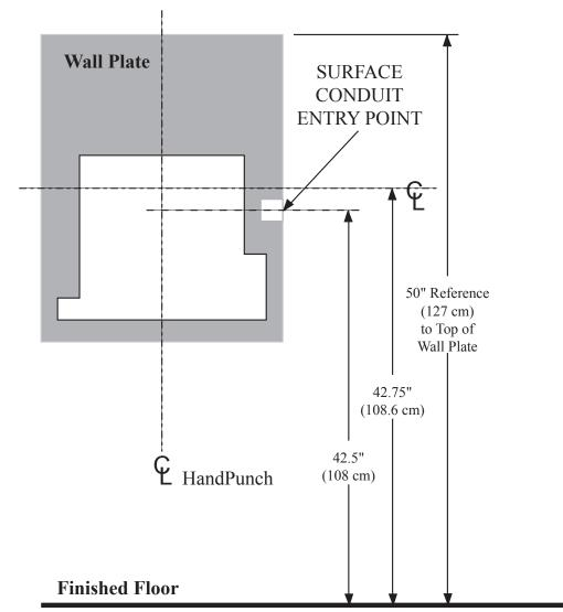
Figure 12-2: HandPunch Wire Routing Layout
