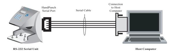
Figure 4-3: Host PC to RS-232 Connection
