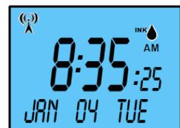
When the clock is powered on, the time is changed, or the **Reset** button is pressed, the clock receiver is enabled to acquire the Atomic Time Synchronization signal, and the indicator will display the triangle tower symbol. Once the correct minutes and seconds [time] is received the curved wave symbol will be displayed with the tower.
