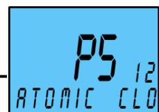
5. Press the **ENTER** button once and the clock will start flashing the current atomic clock setting.
