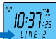
clock will display "**LINE - 2**" for 5 seconds to prompt the user that line 2 is being printed (see example Figure above).
