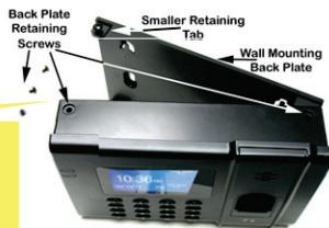
**Next - If desired, wall mount the FPT-80 Biometric Terminal with the supplied mounting hardware.**
